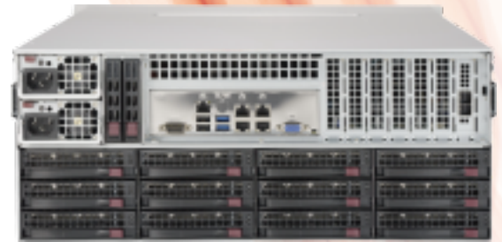
36 Bay | 4U Storage Server
